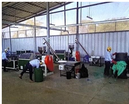
Continuous extrusion lines for bunch bag recycling in Peru.
