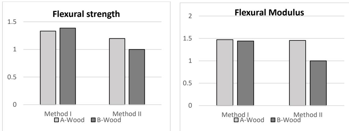
Figure 4. Effect of mixing on the flexural properties of wood fibre composites. The values are normalized with respect to the smaller value.
